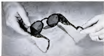
Jointed earpieces make the bows adjustable for size
